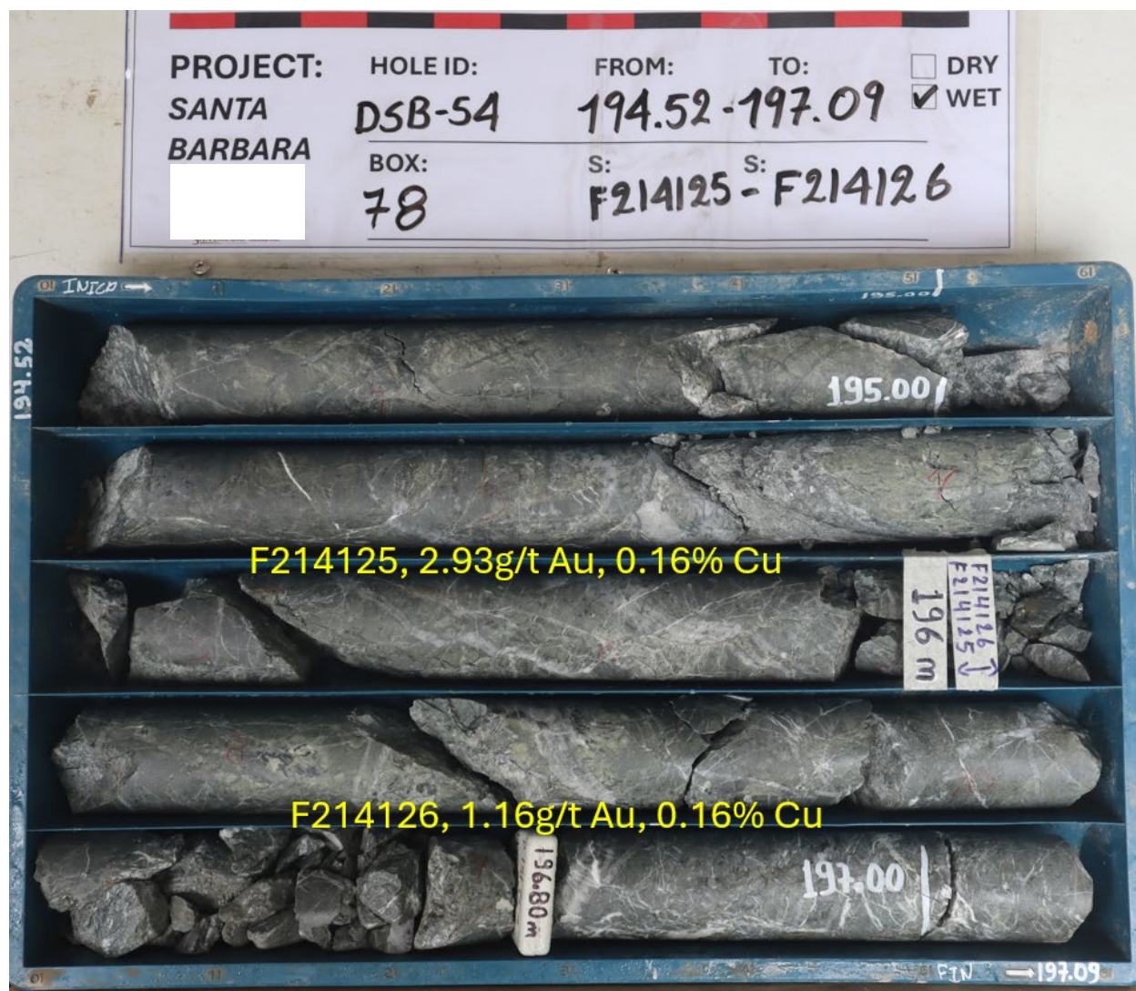
Figure 3: Core photo of DSB-54, Box 78, from 194.52m to 197.09m, mineralized basaltic andesite with milky quartz veining.
