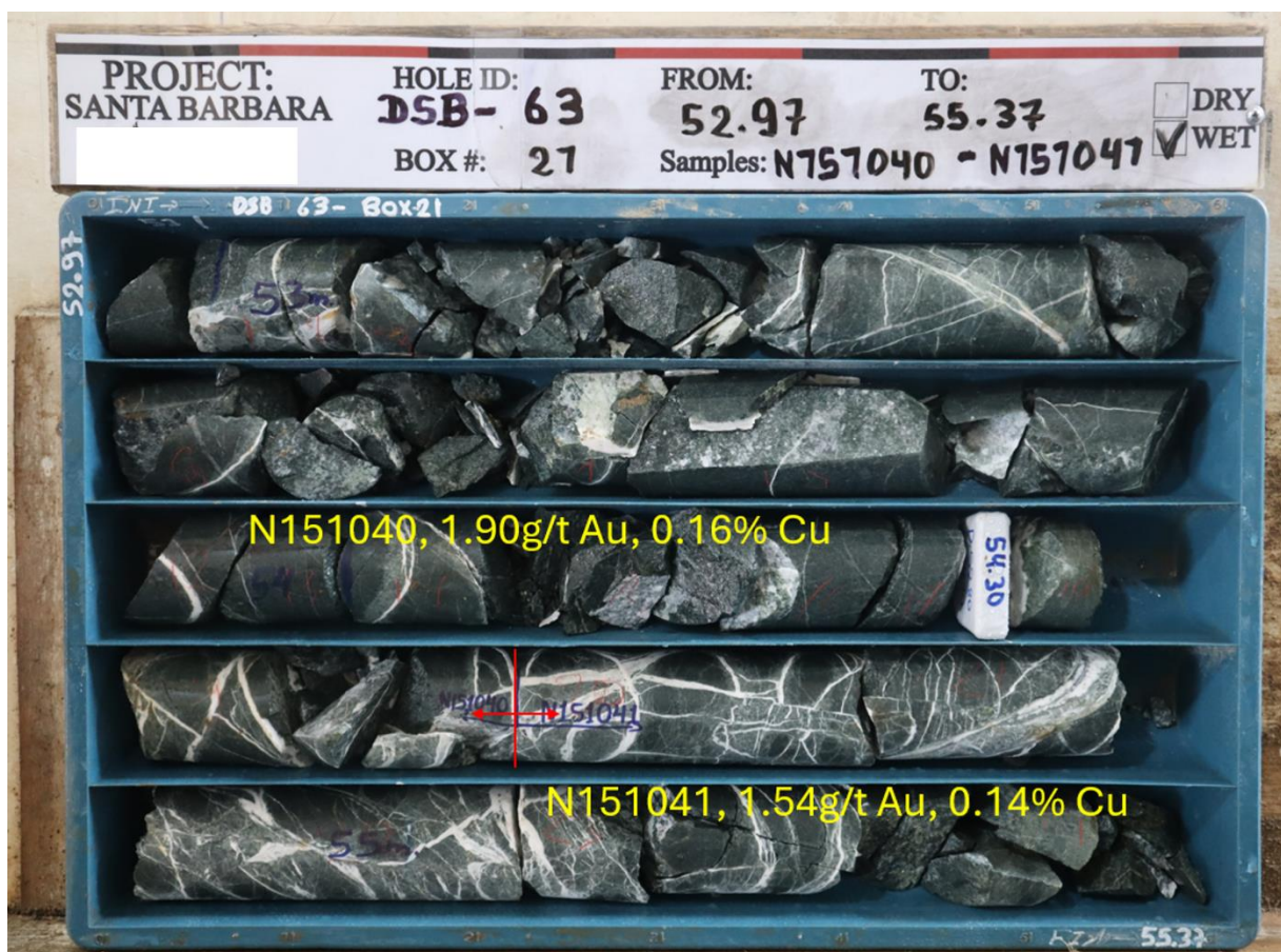
Figure 7: Core photo of DSB-63, Box 27, from 52.97m to 55.37m, mineralized diorite cut by quartz and quartz-calcite veining.
