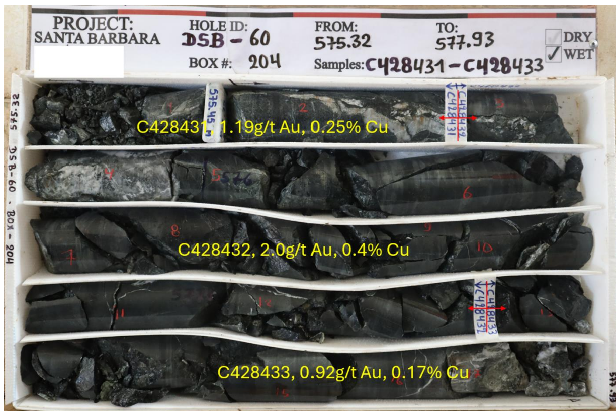
Figure 3: Core photo of DSB-60, Box 204, from 575.32m to 577.93m, mineralized basaltic andesite cut by quartz veining.
