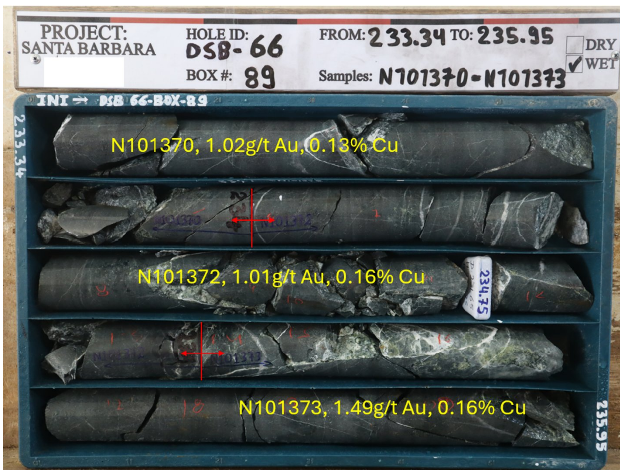
Figure 7: Core photo of DSB-66, Box 89, from 233.34m to 235.95m, mineralized diorite cut by quartz veining.
