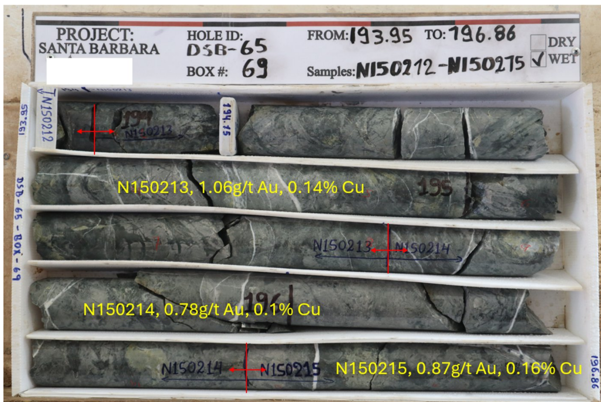
Figure 5: Core photo of DSB-65, Box 69, from 193.95m to 196.86m, mineralized diorite cut by quartz and quartz-calcite veining.
