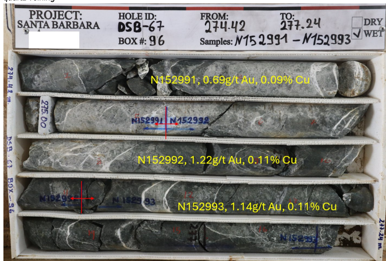
Figure 10: Core photo of DSB-67, Box 96, from 274.42m to 277.24m, mineralized diorite porphyry dyke cut by quartz and quartz-calcite veining
