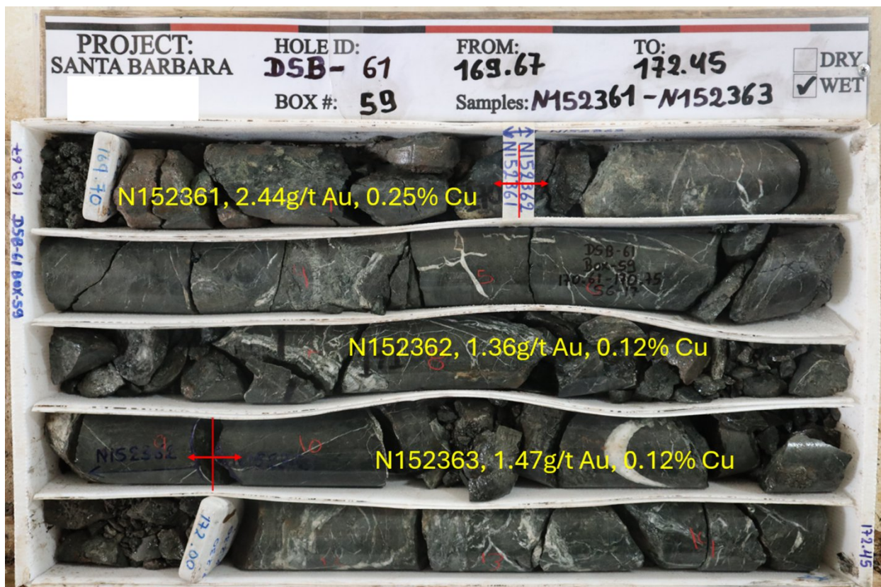
Figure 3: Core photo of DSB-61, Box 59, from 169.67m to 172.45m, mineralized basaltic andesite cut by quartz veining.
